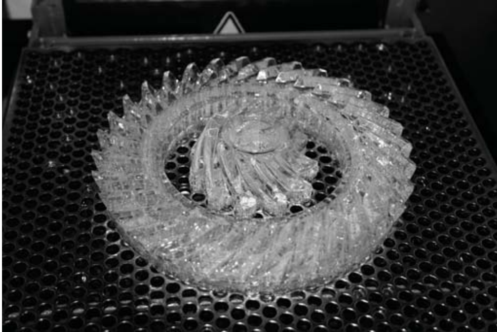
Fig. 2. Finished stereolitography SLA models in UV chamber of SLA-250
