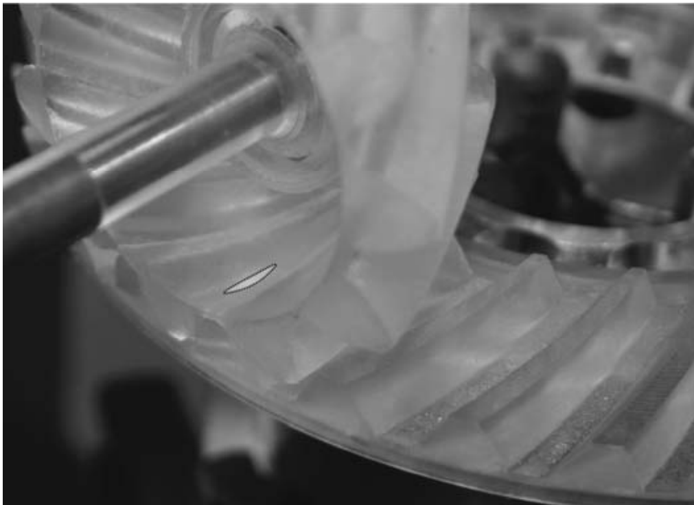
Fig. 4. Contact area (outline with dashed line) between teeth of loaded gear pair with moment
